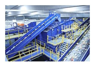
screens or vibrating separators, ACS system with control cabinets.
